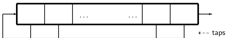
Figure 1.8: Simple graphical representation of an LFSR
